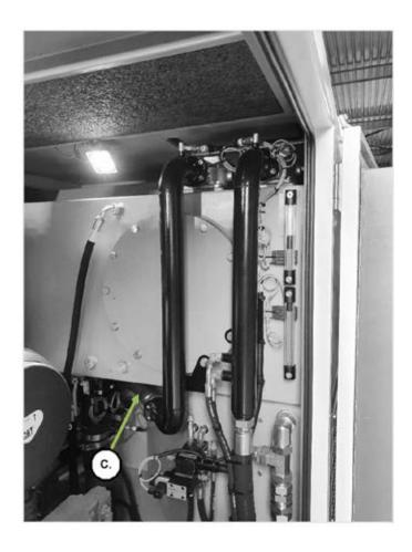
The diesel engine can be drained by opening the drain valve (C) on the engine pan, the manual pump on the frame can be used to drain the oil sump.
