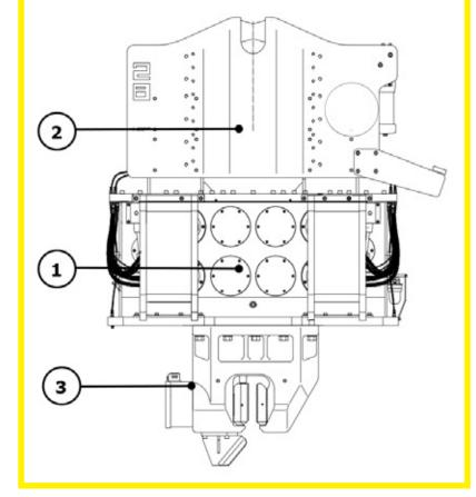
The extraction head contains rubber elements (elastomers) to isolate the vibrations from the vibration case to the crane or pile driving rig. The hammer is attached to the crane with a steel wire rope sling.
