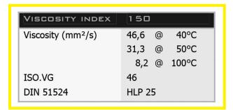
When operating in arctic conditions, it is recommended to use an immersion heater to preheat the oil prior to starting. It may also be necessary in extreme cold or hot climates to use a different viscosity oil which is better adapted to adverse conditions
